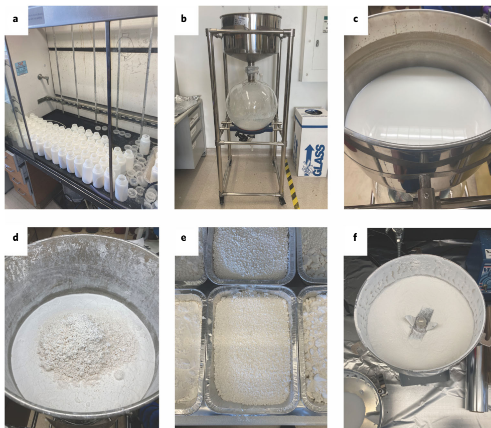
Fig. 5 | Purification of MOF-303 at 3 kg scale. a , Centrifugation with 250 mL open-mouth bottles and drying in the hood. b , 20 L filtration funnel. c , Filtering 10 L of crude MOF-303 reaction mixture. d , White MOF solids obtained after the filtration. e , Collecting 3 kg of MOF powder in aluminum foil pans. f , Grinding aggregates into a fine powder.
